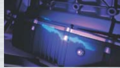
Fluid system leak check
