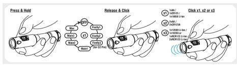
To access the Menu press and hold the switch button (when the flashlight is switched off). It will switch on, go through the all available modes and then switch off again. After switching off, release the button quickly and click it rapidly again. The flashlight will enter the Menu and the LED will flash about 3 times a second.
