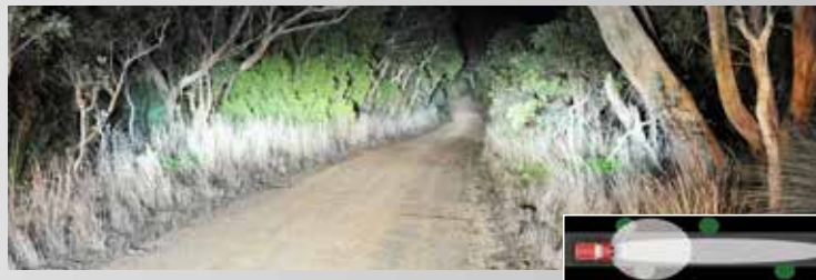
FIGURE 3 Lightforce Genesis 50W HID 5000K • 1 X Lightforce Spot Filter & 1 X Lightforce Combo Filter
