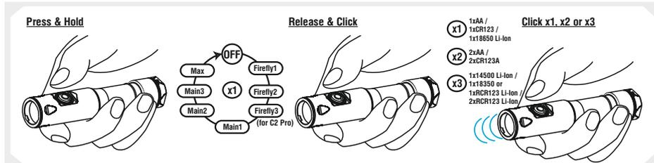
To access the Menu press and hold the switch button (when the flashlight is switched off). It will switch on, go through the all available modes and then switch off again. After switching off, release the button quickly and click it rapidly again. The flashlight will enter the Menu and the LED will flash about 3 times a second.
