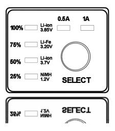
Connect the 5V input port with USB cable, the LED indictor of 0.5A on when no battery is inserted. When broken battery inserted, the charge will have no any response.
